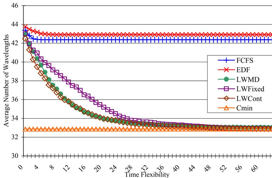
**Figure 4. The average number of wavelengths so there is no blocking.**
