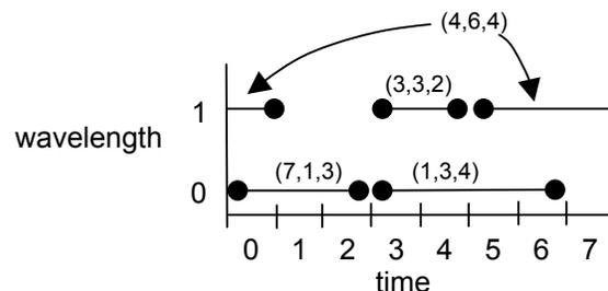
**Figure 1. An assignment of a batch of four lightpath requests.**
